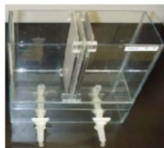
Fig. 2 Device of electrolyzed water production
