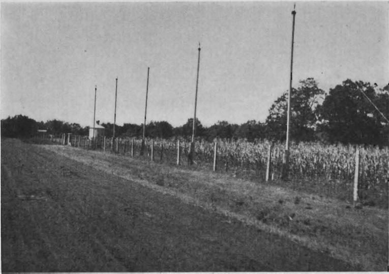
Fig. 2. Utilization of atmospheric electricity for crops, Agronomy Farm, 1930, 1931, 1932. South view of experimental field showing the five elevated brushes and instrument house.
