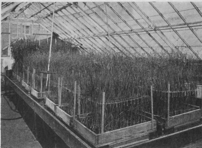
Fig. 5. Earth cell test with oats, 1932. Alternate flats are equipped with the copper-zinc electrode combination. Two lots have additional current supplied by a dry cell. The high fertility lots are at the far end of the bench.
