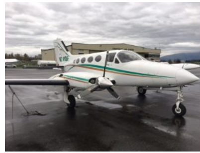
A turboprop sits on the tarmac. These pressurized twin-engine airplanes carry both hygroscopic and glaciogenic flares to use for cloud seeding. (Photo courtesy of Gary Walker/SOAR)
