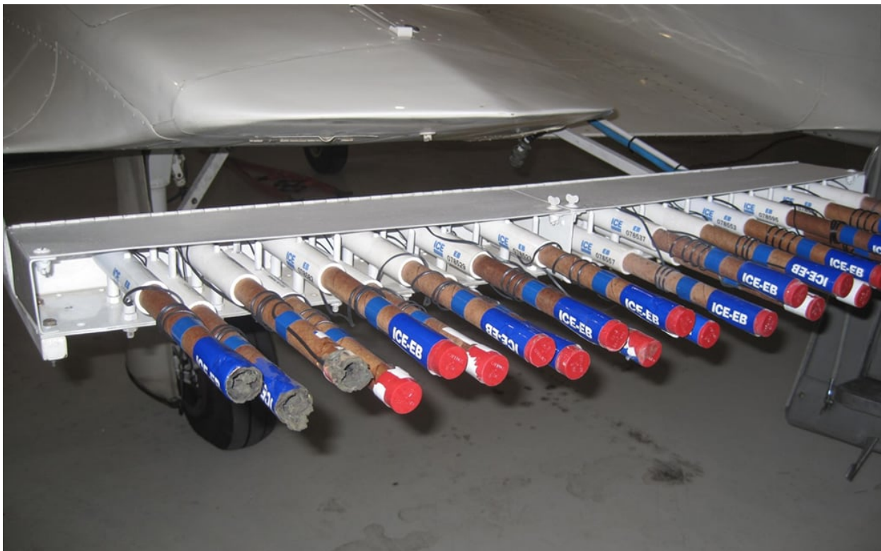
A rack of glaciogenic flares is loaded onto a rack on the wing of a plane. These flares are used to create snow in winter months. (Photo courtesy of Gary Walker/SOAR)
