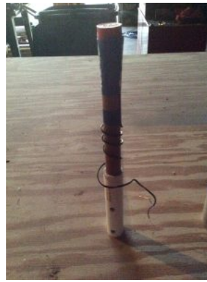
A glaciogenic flare rests on a wooden work bench. These flares are used to create snow in winter months through cloud seeding. (Photo courtesy of Gary Walker/SOAR)
