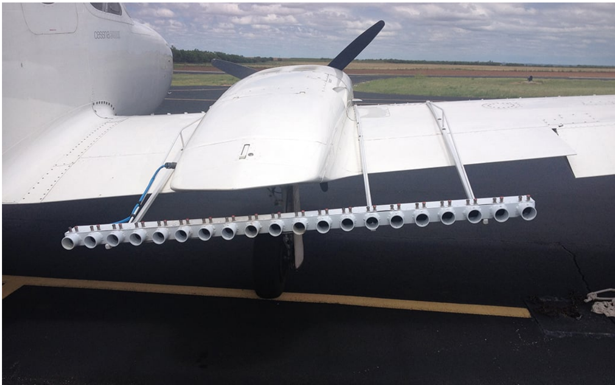
An empty rack for flares sits on the wing of a twin-engine airplane. (Photo courtesy of Gary Walker/SOAR)
