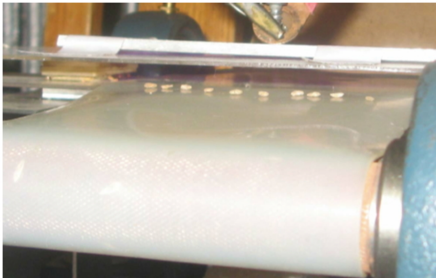
Figure 2. Process of treating seeds by plasma device.
